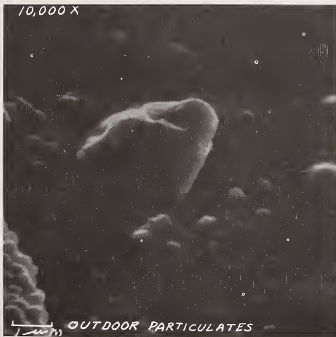
Figure 8. 10,000X SEM of impaction area of smog sample (same as in fig. 7).
